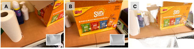
Figure 1: Illustration of 3D pointcloud generation steps. We use RGB+D (A, B—Small box at the bottom right indicates Depth image) image captures to generate 3D point clouds (C) and associate the transformational information with the detected/class instance of Gemini 2.5-Flash. We adapt the data collection pipeline of Explainable XR [2].
